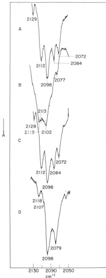
Fig. 17. The cyanide stretching vibrational bands in  $[\text{Cr}(\text{en})_3][\text{Ni}(\text{CN})_5] \cdot 1.5 \text{H}_2\text{O}$ : A, at 78 K and ambient pressure; B, at 78 K and ca. 7 kbar; C, at 78 K and ambient pressure after release of high pressure. Spectrum D is that of  $[\text{Cr}(\text{en})_3][\text{Ni}(\text{CN})_5]$  at ambient temperature and pressure [249]. (Figure reproduced through the courtesy of the authors and the American Chemical Society, Washington, D.C.)
